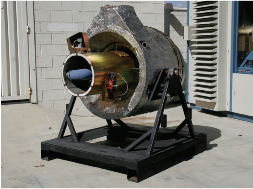
A beta version of the new C200 microturbine is shown during test at the Capstone facility. The new turbine includes features from the company's C30 and C65 microturbines.
